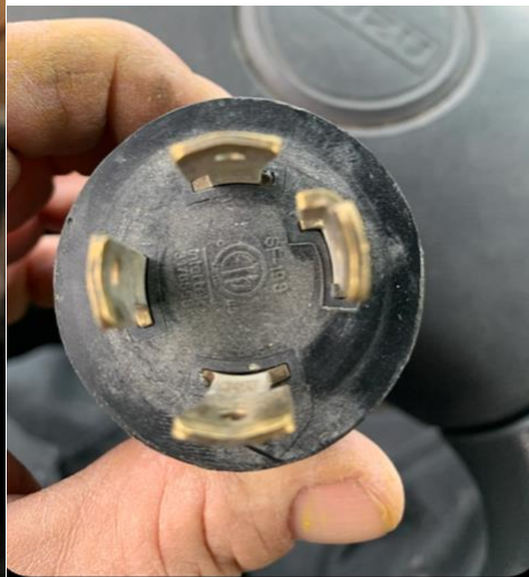
This is for the small grinder 220 vol Single phase requires a 30 amp breaker
