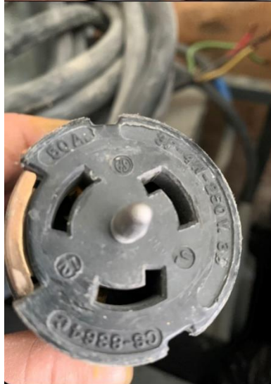
This one is the big grinder the requirements are 208 3 phase 60 amp breaker
